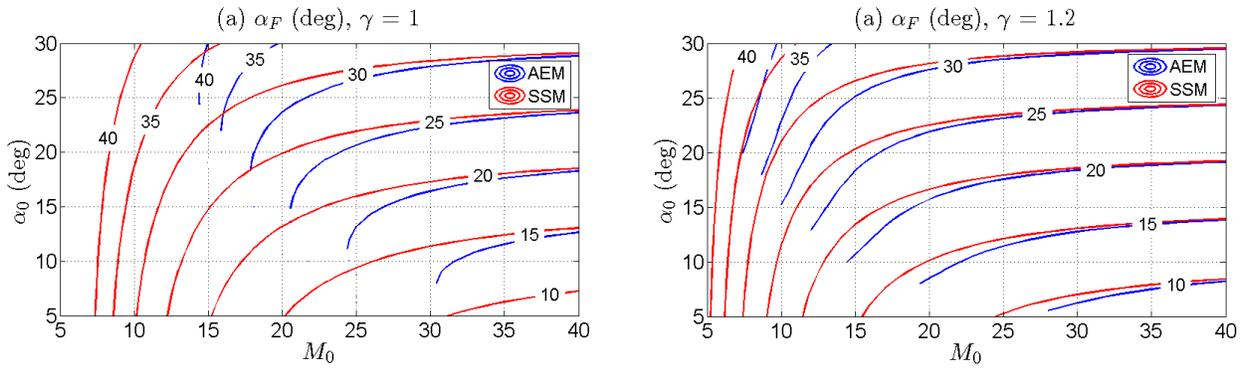
**Figure 9.** Far field divergence angle contour plot for  $\gamma = 1$  (a) and  $\gamma = 1.2$  (b), calculated using the two approximated methods: AEM first order (blue lines) and SSM (red lines). AEM first order solution shown only when within its convergence region.
