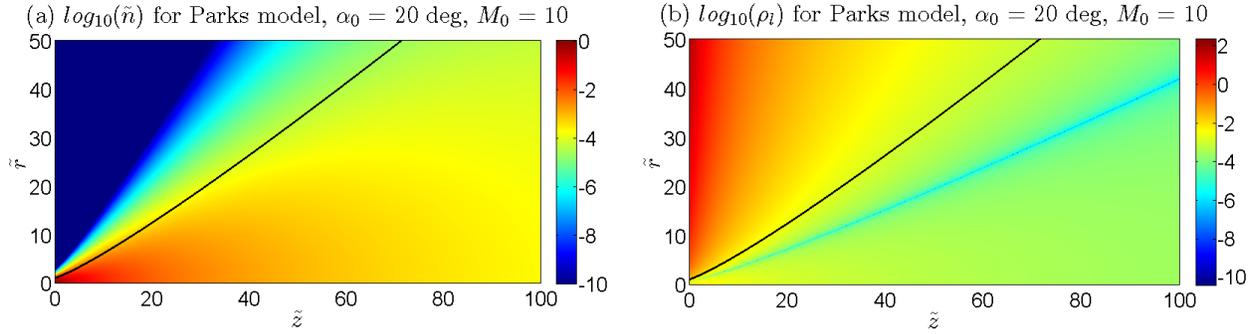
Figure 5. Density plot for the Parks-Katz model (a) and the corresponding local relative error in the axial momentum equation (b). The 95% ion current line is shown as a solid black line in both a) and b).
