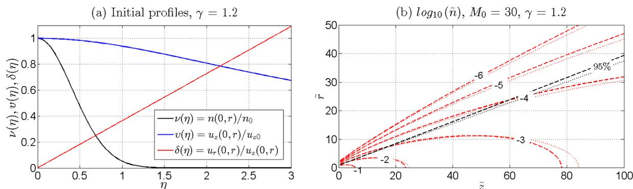
**Figure 2.** (a) Initial normalized profiles for density, axial velocity and divergence for  $\alpha_0 = 20$  deg,  $\gamma = 1.2$ , a Gaussian density profile and a conical velocity field. (b) Corresponding plasma density (red lines) and 95% ion current streamlines (black lines) for a  $M_0 = 30$  flow for both the zeroth (dotted line) and first order (dashed line) solutions.
