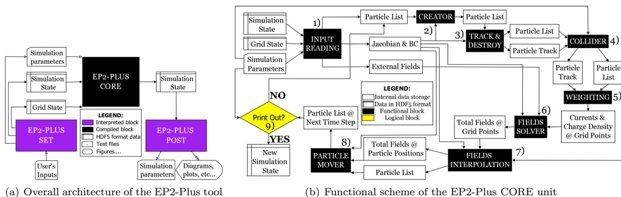
Figure 10. EP2-Plus overall architecture (a) and block scheme of the CORE unit (b)
