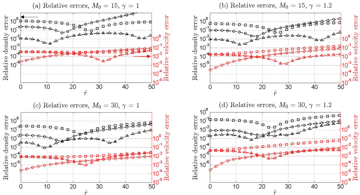
Figure 7. Relative errors with respect to the MOC solution in density (black lines) and velocity (red lines) at  $\tilde{z}=100$  as a function of the radius. Different combinations of  $M_0$  and  $\gamma$  are considered: (a)  $M_0 = 15$ ,  $\gamma = 1$ , (b)  $M_0 = 15$ ,  $\gamma = 1.2$ , (c)  $M_0 = 30$ ,  $\gamma = 1$ , (d)  $M_0 = 30$ ,  $\gamma = 1.2$ . Different methods are shown: AEM zeroth order (squares), AEM first order (circles) and SSM (triangles).
