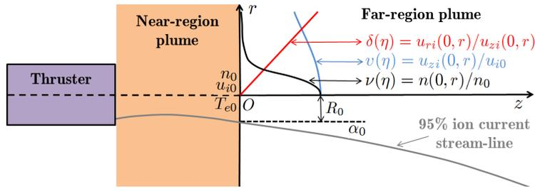
Figure 1. Schematic of a plasma plume and its different regions. The reference plane that serves as the initial condition for the far-region plume is a few thruster radii downstream from the plasma source exit.
