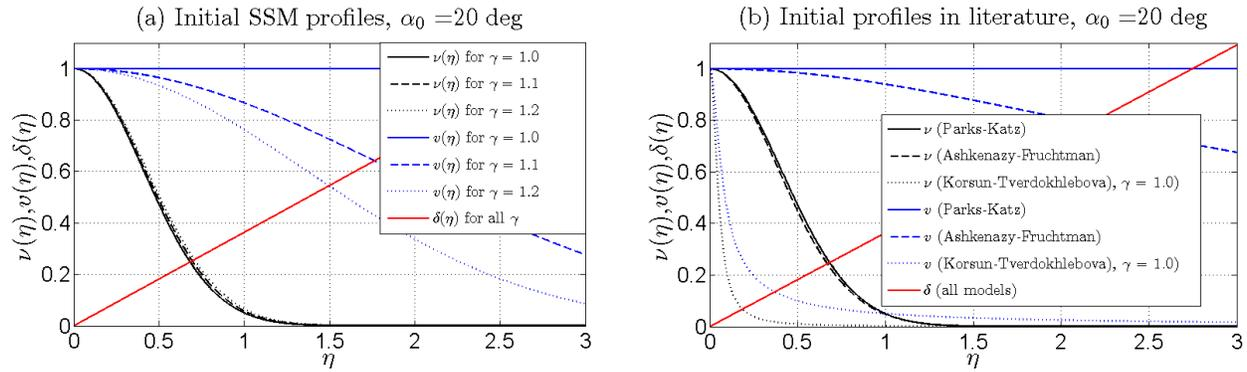
Figure 4. SSM initial profiles: dependence on  $\gamma$  (a) for a Gaussian density profile. Initial profiles considered by several authors (b). Ashkenazy-Fruchtman profile has been obtained with the choice  $k = \tan^2(\alpha_0)$ .
