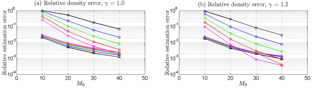
**Figure 8.** Relative error in the density estimation at  $\tilde{z} = 100$ ,  $\tilde{r} = 0$  for  $\gamma = 1.0$  (a) and  $1.2$  (b) for both the first order AEM (circles) and the SSM (triangles).  $\alpha_0 = 10$  deg (black lines),  $15$  deg (blue lines),  $20$  deg (green lines),  $25$  deg (red lines),  $30$  deg (magenta lines).
