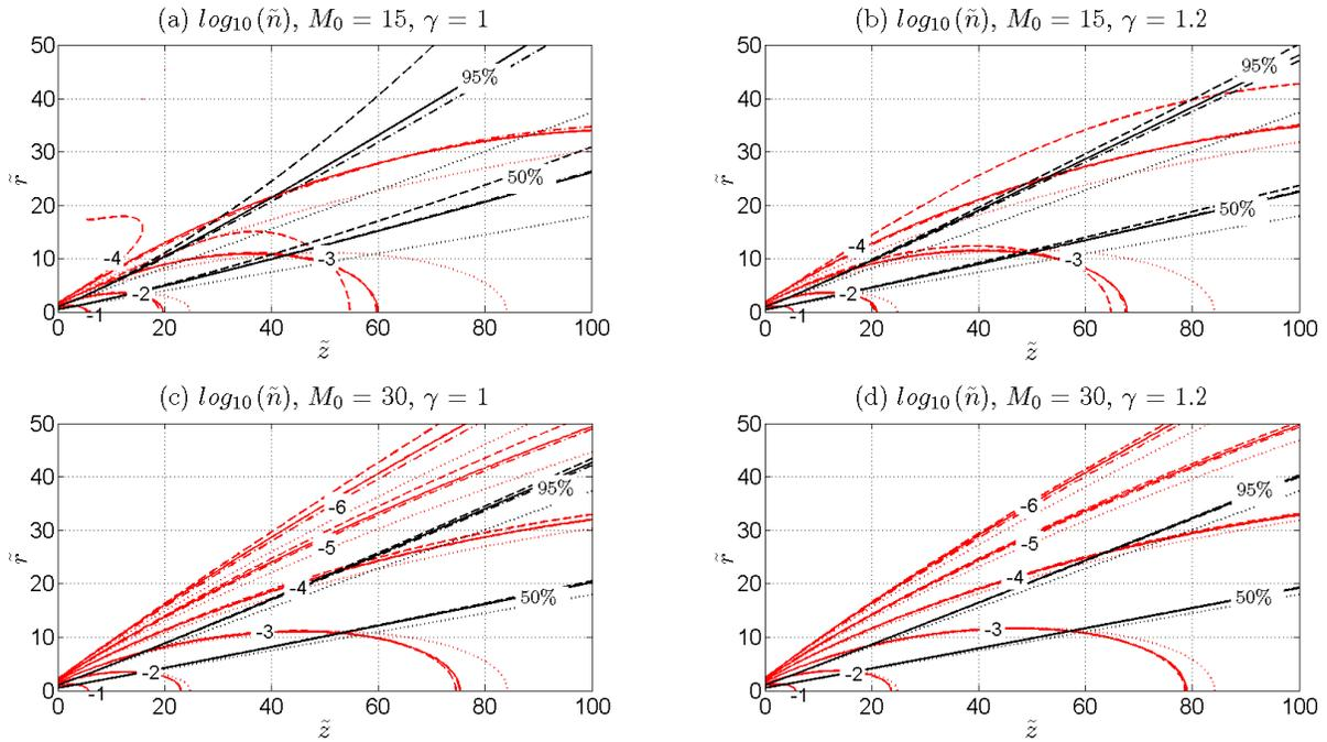
Figure 6. Density contour plot (red lines) and 50-95% ion current lines (black lines) for  $\alpha_0 = 20$  deg and different combinations of  $M_0$  and  $\gamma$ : (a)  $M_0 = 15$ ,  $\gamma = 1$ , (b)  $M_0 = 15$ ,  $\gamma = 1.2$ , (c)  $M_0 = 30$ ,  $\gamma = 1$ , (d)  $M_0 = 30$ ,  $\gamma = 1.2$ . Different methods are shown: AEM zeroth order (dotted lines), AEM first order (dashed lines), SSM (dash-dot lines) and MOC (solid lines).
